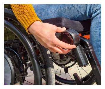
One click on the control unit is all it takes to switch to Cruise mode while driving.
