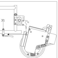
Slide the lower bolt [1] of the viamobil into the lower holder [31] on the wheelchair until it reaches the stop.
