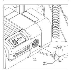
• Insert the plug of the control unit [21] into the socket [11] on the battery pack. The connection is secured automatically and conveniently by magnetic force.
