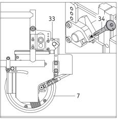
• Close the forks [33] on both sides with the quickpin [34] as soon as the upper bolt [3] of the viamobil is seated in the fork [33] (see also chapter 2.2).
