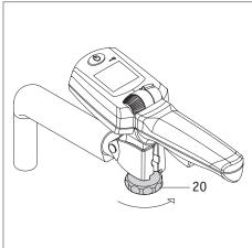
• Turn the locking wheel [20] clockwise until the control unit [13] is seated firmly in the holder [22].
