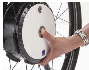
The wheel can be removed by pressing the button on the quick-release axle and pulling the wheel off – a perfect example of built-in multifunctionality.
