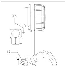
Removing the control unit
