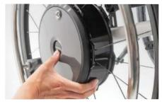
The wheel can be removed by pressing the button on the quick-release axle and pulling the wheel off.
